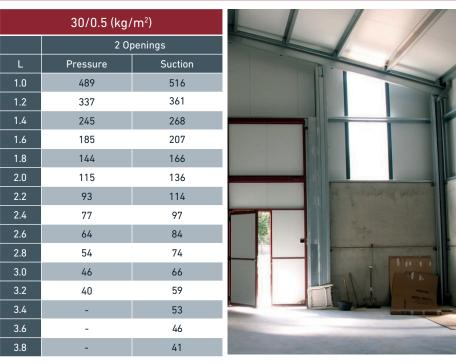
Permissible service loads, uniformly distributed in kg/m<sup>2</sup>. The tables have been obtained based on a calculation methodology established in accordance with the provisions of the EAE-2012 standard and the EC-3, considering only the upper steel sheet as a structural element. These results comply with the Ultimate Limit States of normal and tangential stresses prescribed in said standards and with a limitation of the Serviceability Limit State for deformations of L/200.
