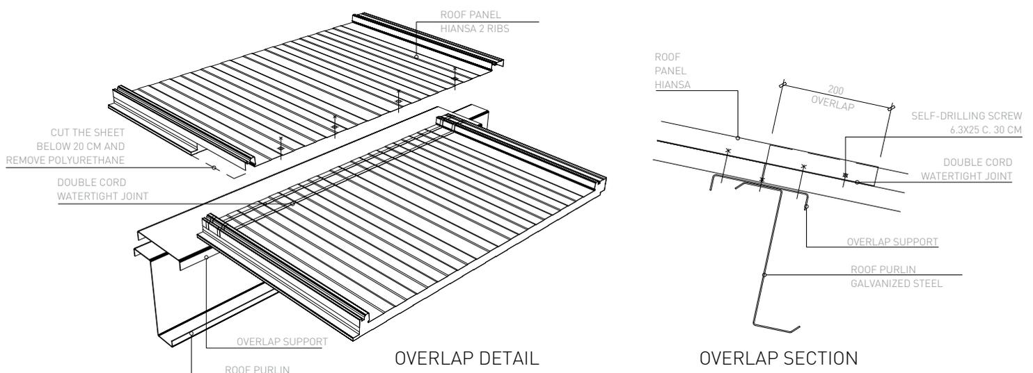
To resolve the overlap between the flashings of the panel, proceed as indicated in the following figures, taking into account to never perform the panel overlap at the same point as the flashing overlap.
