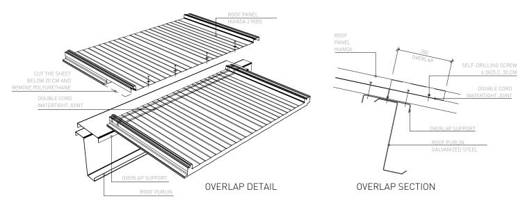
To resolve the overlap between the flashings of the panel, proceed as indicated in the following figures, taking into account to never perform the panel overlap at the same point as the flashing overlap.
